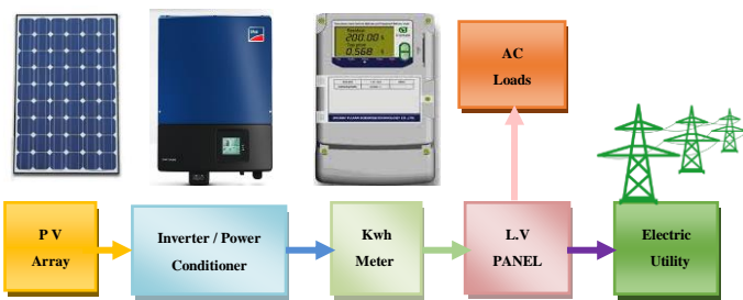
Fig. 3. Grid-connected or utility-interactive PV systems
