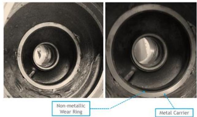
Fig. 5. Non-metallic installed in metal carrier
